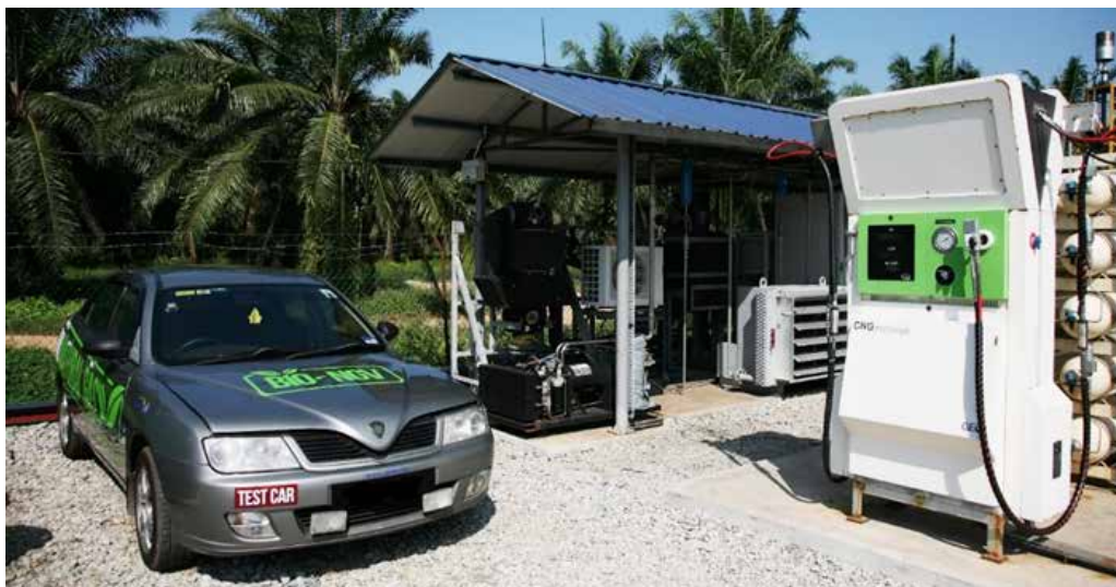
Figure 4.17 Bio-natural gas vehicle prototype and prototype fuelling pump
