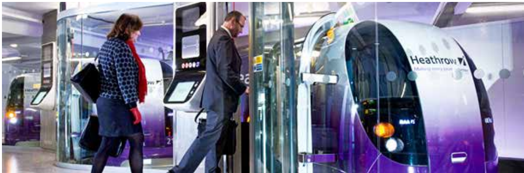
Figure 4.9 ULTra PRT that facilitates the journey between the stations at the business car parks and Terminal 5
