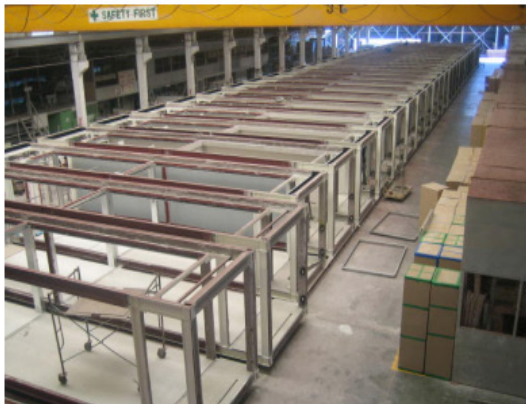
Figure 4.2 Modular Unit Construction
