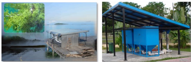
Figure 8.16 Solar drying system for agricultural and marine products
