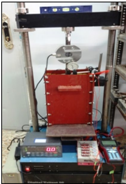
Figure 4. Set-up of the physical model with the loading machine.
