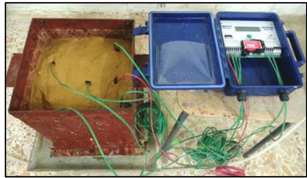
Figure 5. Five calibrated sensors are embedded in the soil bed to monitor the soil saturation.
