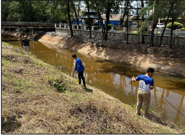
Figure 2. Setting up resistivity survey for line L1, parallel to the shoreline.
