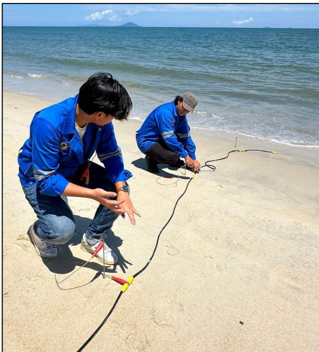
Figure 3. Setting up resistivity survey line L2, perpendicular to the shoreline.
