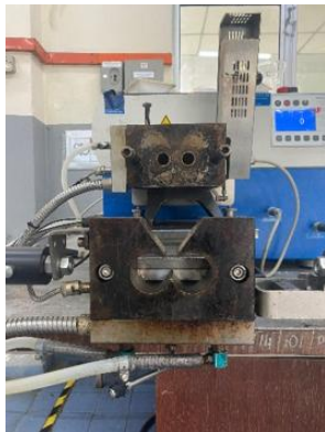
Figure 1. Brabender melt mixer .
