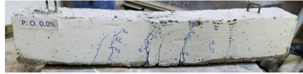
Figure 15. Beam P.O.0.0% Failure
