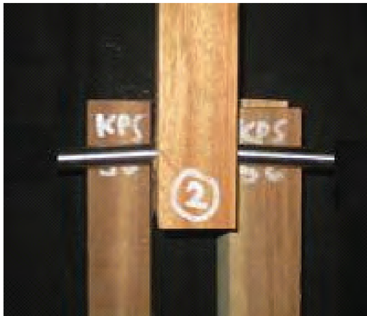
Figure 7. Double shear joint after test — failure mode III s for steel dowel.
