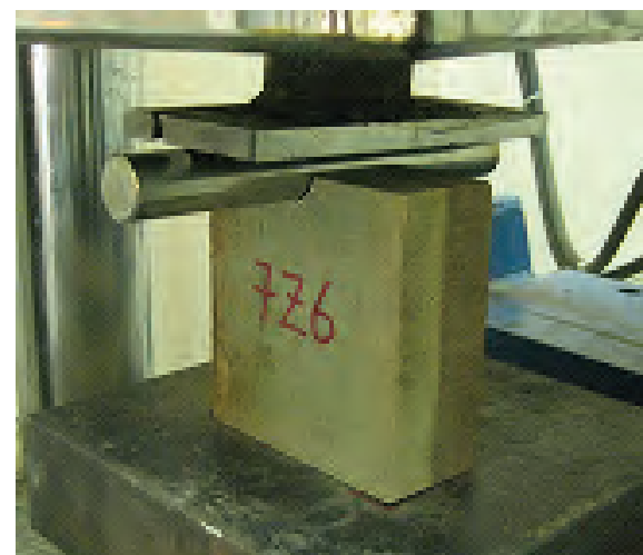
Figure 2. Dowel bearing test set-up: (a) Schematic diagram and (b) Actual test set up.
