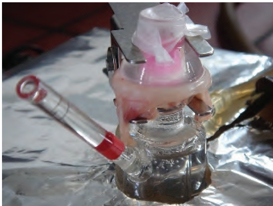
Figure 4. Ex-vivo permeability model: Franz Cell.
