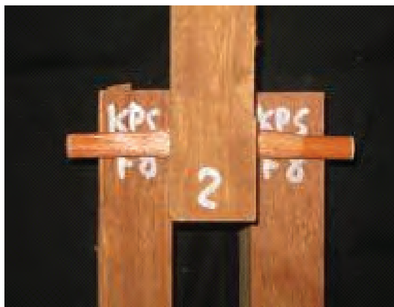
Figure 8. Double shear joint after test — failure mode IV for GFRP dowel.
