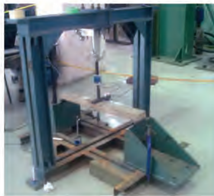
Figure 3. Bending test set-up; showing schematic diagram and actual test set up.
