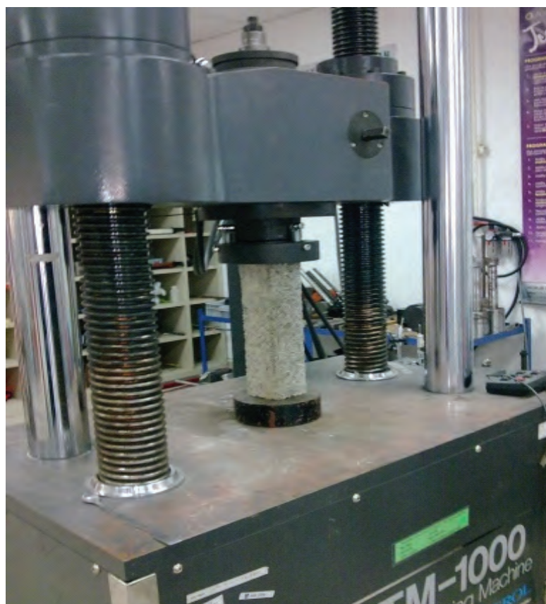
Figure 2. Compression test set-up.
