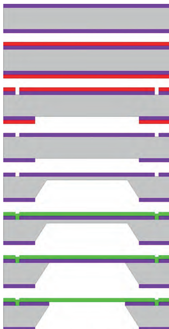
Figure 2. Step process fabrication of polyimide membrane.
