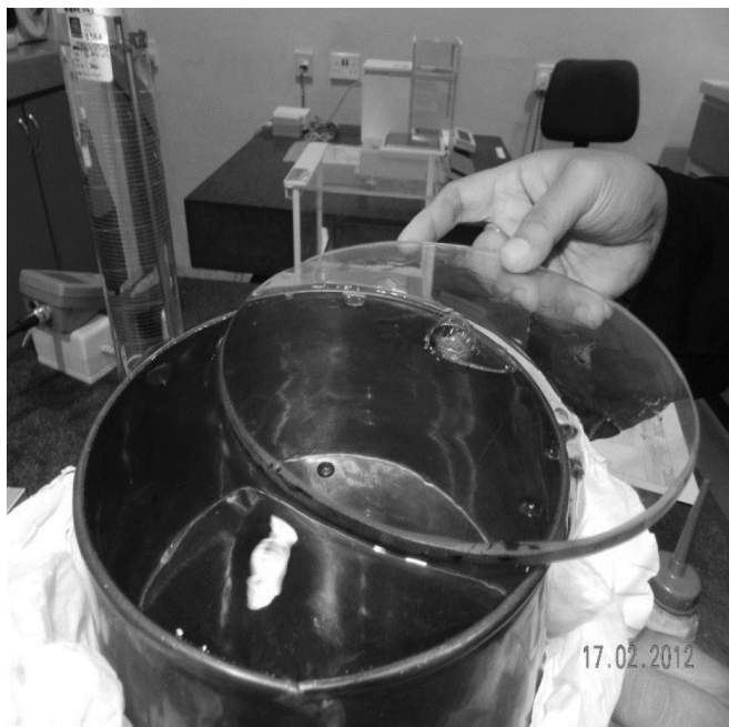
Figure 7. The use of slicker plate to level water in the gravimetric calibration
