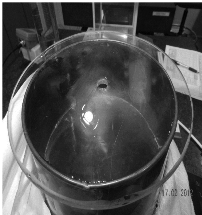
Figure 6. The use of slicker plate to level water in the gravimetric calibration
