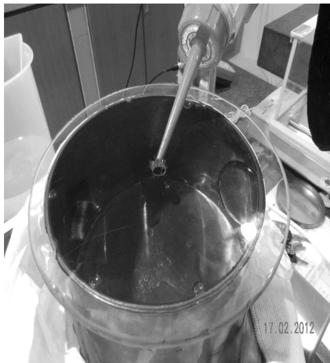
Figure 5. The use of slicker plate to level water in the gravimetric calibration
