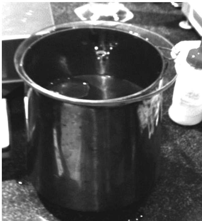
Figure 3. The use of slicker plate to level water in the volumetric calibration
