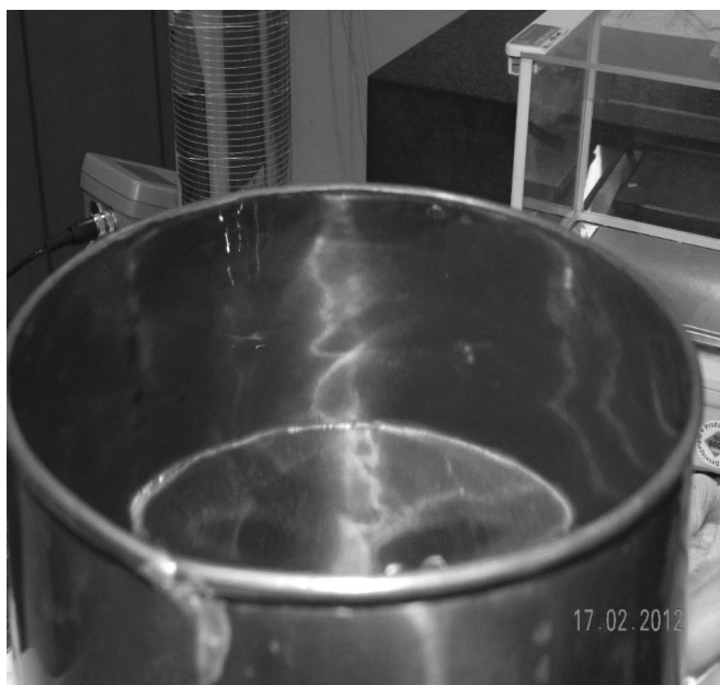
Figure 8. Water is used for the gravimetric calibration of gantang Baghdad
