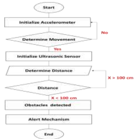
Figure 4: Flowchart design of Obstacle Detection system
