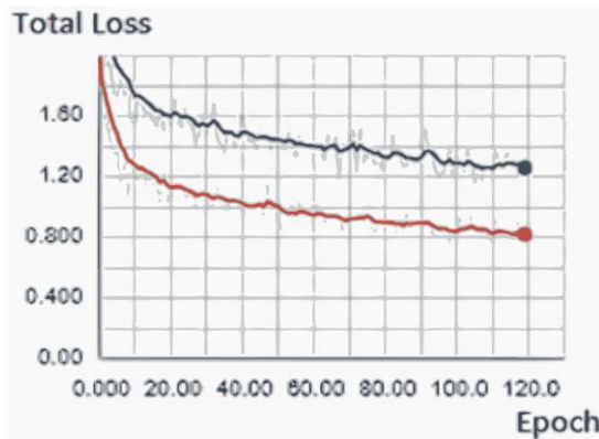
Figure 9. Total loss per epoch for Mask R-CNN before Edge Agreement Head was applied (orange) and Mask R-CNN after Edge Agreement Head was applied (blue)
