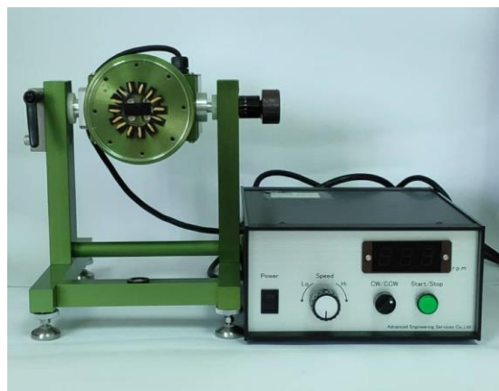
Figure 1. The experimental set-up of the clinorotation of rice seeds MR 219
