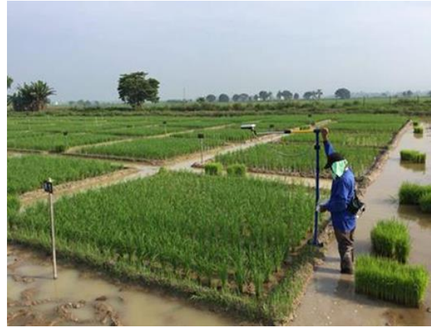
Figure 2. Crop Circle ACS-430 sensor mounted on customized pole-holder during data acquisition on studied subplot
