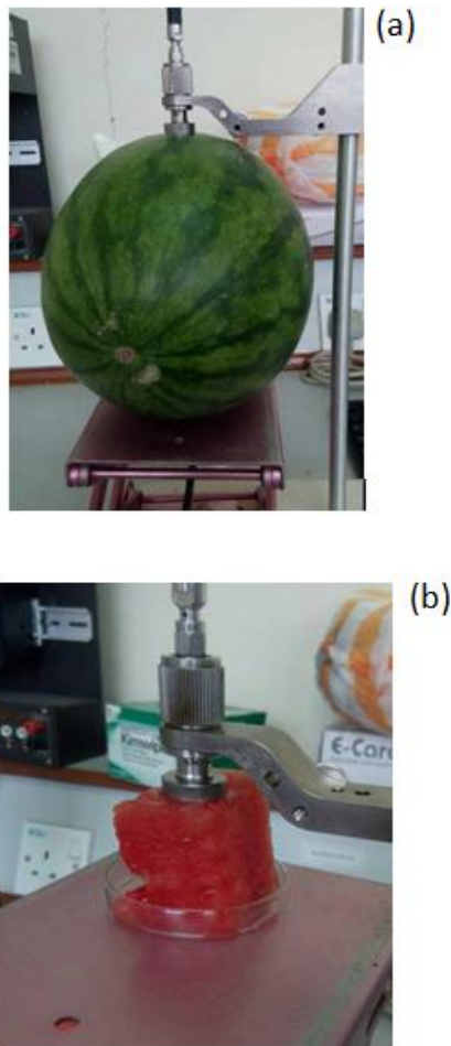
Figure 3. Dielectric properties measurement at the (a) surface, and (b) internal tissue of watermelon samples
