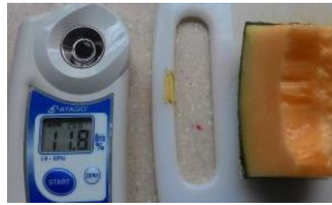
Figure 2. Pocket Refractometer to measure Brix level of rockmelon
