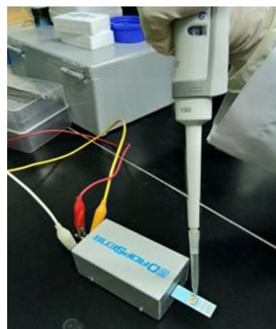
Figure 1. Electrochemical analysis on gold SPE is performed by dropping a 150 \mu L of redox solution covering all electrodes surface
