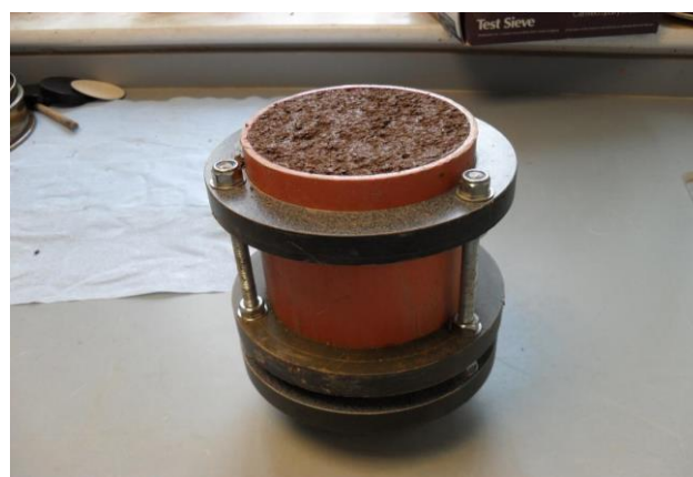
Figure 4. Soil core sample in the plastic core is ready to slice
