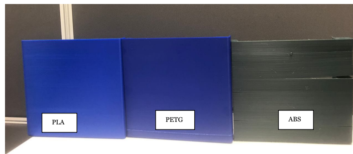
Figure 14. 3D Printed designs after 24 hours of applying disinfectant solution
