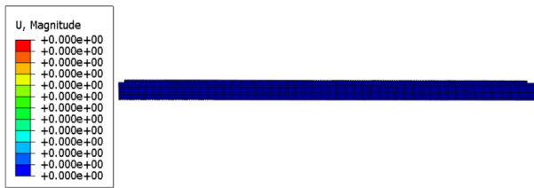
Figure 13. Vertical displacement of SSB before expose to fire and load
