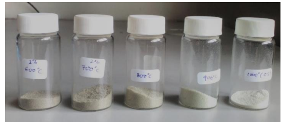
Figure 1. Pictures of samples heated at 600, 700, 800, 900, and 1000 °C (from right to left)
