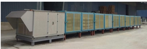
Figure 2. Drying chamber that can accommodate up to 10 pallets of sericite mica
