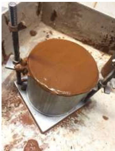
Figure 6. Water saturated for permeability test for sample S1. Other samples do not able to proceed due to its slurry condition when added with more water
