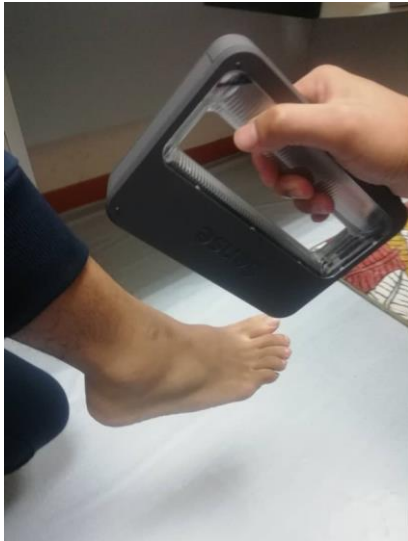
Figure 2. Leg scanning in the progress using 3D scanner (Sense)
