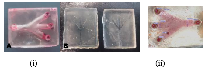
Figure 13. 3D printed microflow cytometer device (i) device with different channel size (ii) red liquid injected into channels
